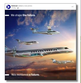
Embraer o 10 November 2 A Moumber 2021 . Our new 9-seat sustainable concept Energia Electric generates zero carbon emissions and is very quiet. It has two super-efficient contra-rotating propellers. The high-aspect ratio wing is inspired by gliders. Meet the whole #EnergiaFamily at https://embr.cc/ytG8 #Embra #ESG #WeAr
