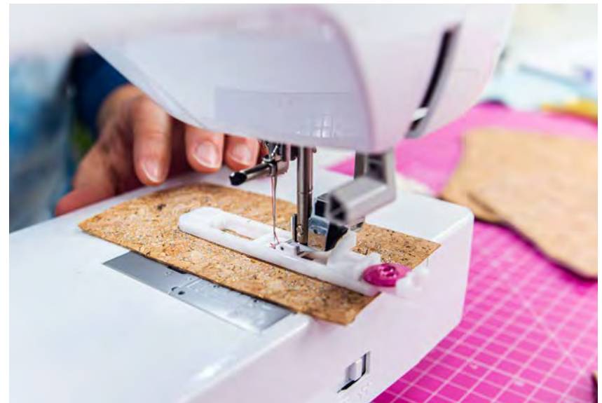
One-step buttonhole sewing
